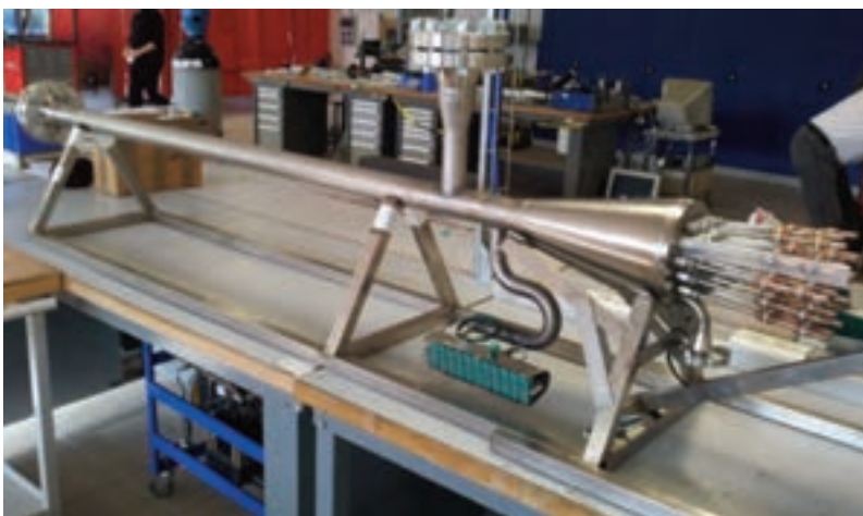
Fuel Pin Bundle Simulator, Impianto NACIE
