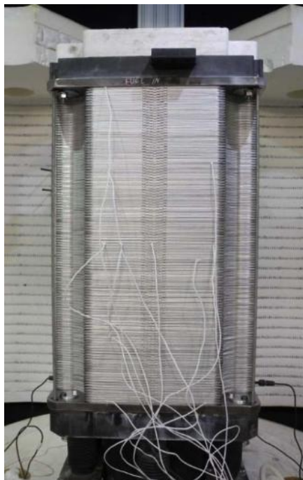
Figure 16. Baseline FCE/Versa SOFC stack building block: Cell size 25x25 cm 2 , 120 cells, 68% fuel utilization, 25-70% in-stack reforming, around 16 kW gross DC electrical power [source: www.netl.doe.gov ]
