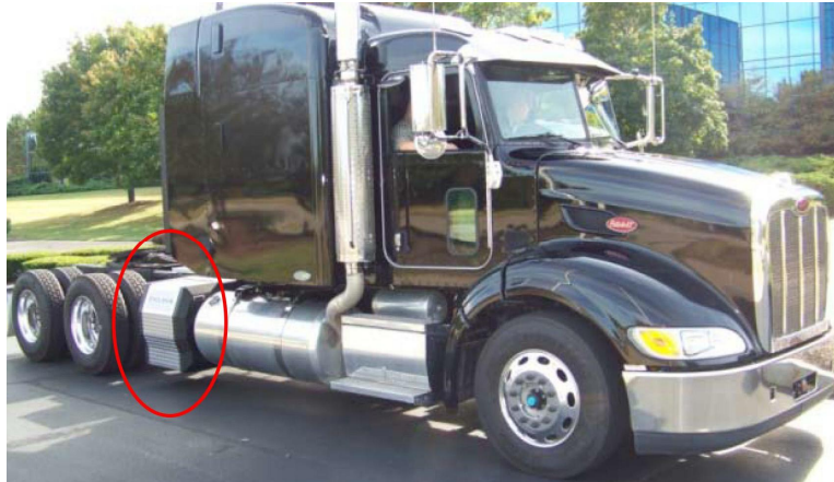
Figure 7. A demonstration model of the Delphi APU on-board of a commercial truck [sources: Delphi, Proceedings of Fuel Cell Seminar 2011 and DoE Peer Review 2012]
