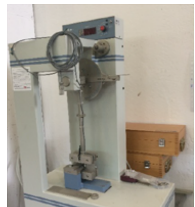
Pendulum CEAST (Instron) with 25 Joule hammer
