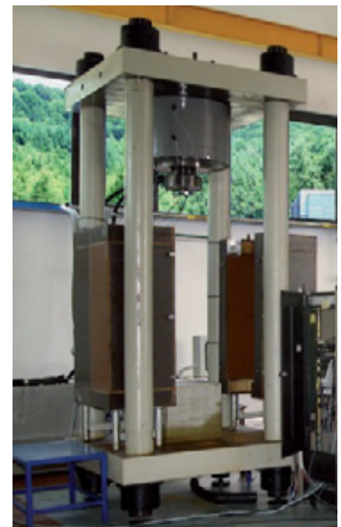
Hydraulic machine for compressive fatigue designed and developed by ENEA, 8000 kN size
