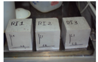
Concrete specimens for qualification tests
