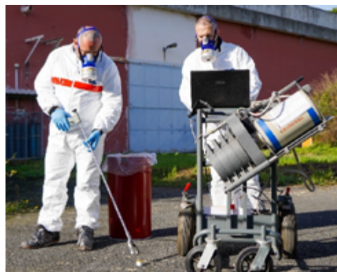
In situ gamma spectrometry for detection and quantification of gamma emitters at the client's premises
