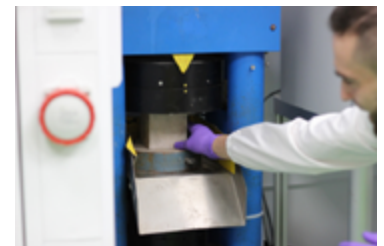
Compressive strenght test
