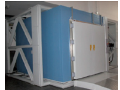
Climatic chamber for thermal cycling tests.
