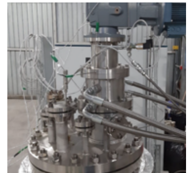
BID1 facility: detail of the cover flange and penetrations
