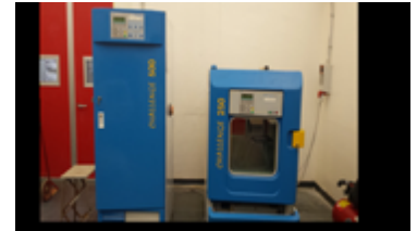
Climatic chambers for the curing of cementitious specimens and thermal cycle tests
