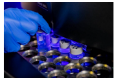
Liquid Scintillation Counting to quantify the presence of beta emitters
