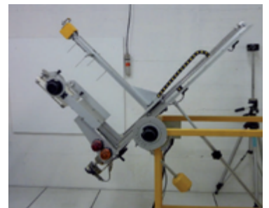
Angular irradiation of personal dosimeters with beta sources
