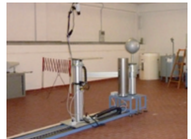
Calibration centre for ionizing radiation (neutron irradiation facility)
