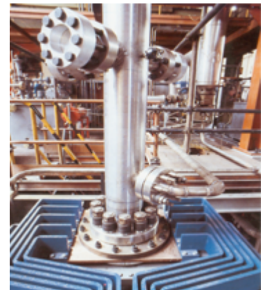
SPES-2 experimental facility: upper head of the power channel (power: 5 MW, n. 97 heated rods)
