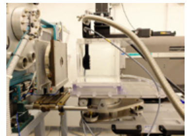
National Dosimetry Standards for Medium Energy X-Ray Radiation for the quantity absorbed dose to water (foreground) and air kerma (background)
