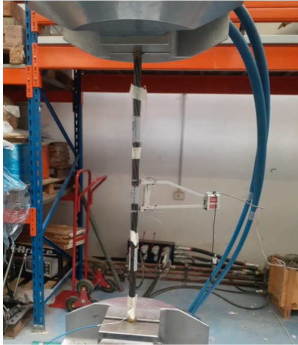
Figure 70. Extensometer positioning for direct strain measurement
