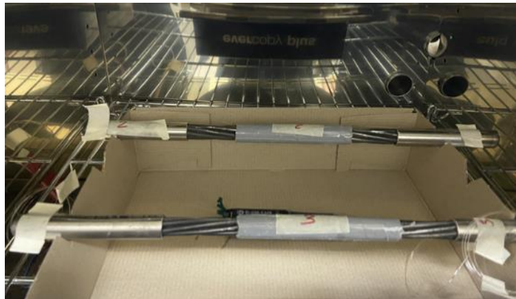
Figure 24. The bonded smart saddles on the strands in the oven.
