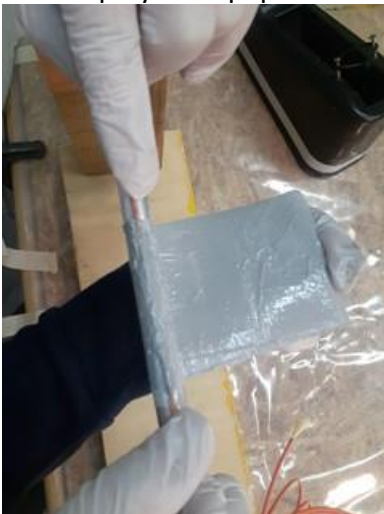
a) FBG + coating gluing to polyester paper
