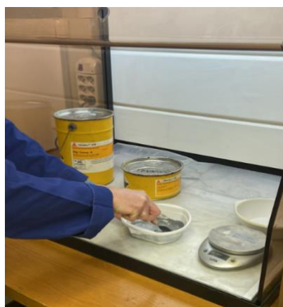
Figure 14. Production of the SIKADUR 330 epoxy resin.
