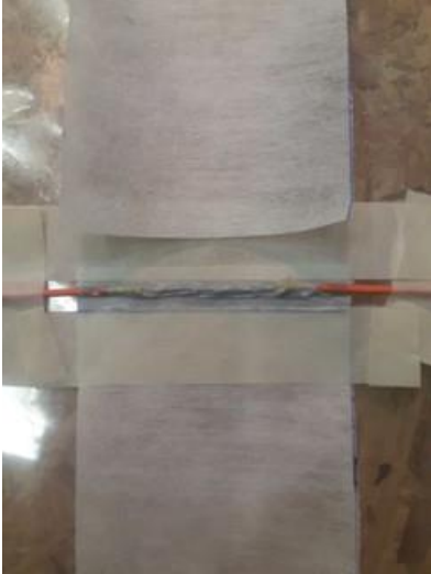
a) FBG + coating gluing to polyester paper
