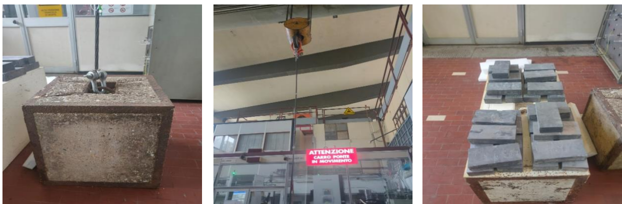
Figure 64. On the left: attachment of the heavy to the strand; in the middle: tensioning of the cable using the overhead crane; at right: progressive increase in load using lead blocks of 11.34 kg each.
