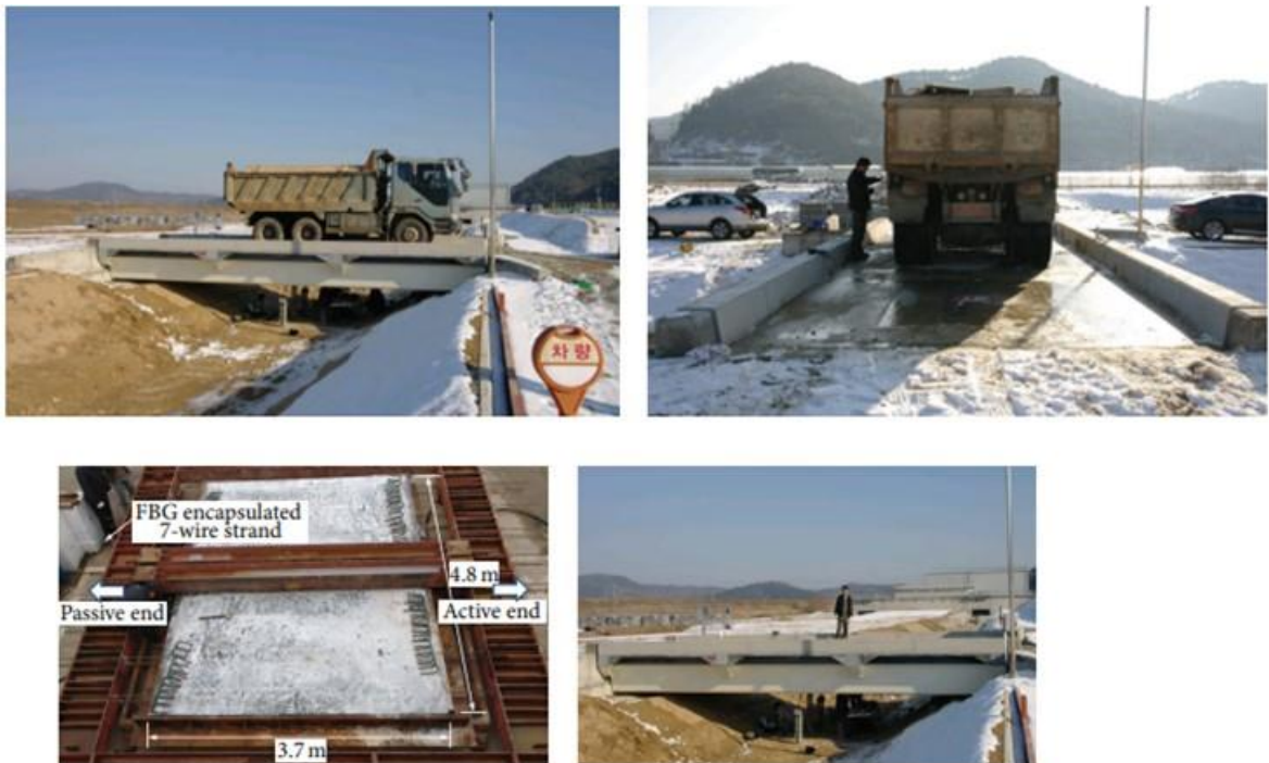
d) Bridge load test and strand internal force monitoring using FBG sensors in Korea (J.-m. Kim, Kim, Choi, & Park, 2016)
