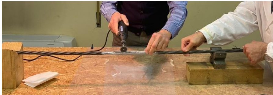
Figure 20. Cutting a small part of smart saddle after curing.
