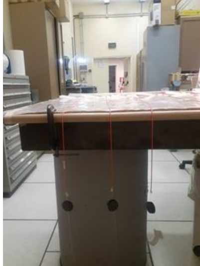
b) Applying the weight
