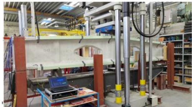
b) Bridge Girder damage assessment using FBG strain data (Anastasopoulos et al., 2018)
