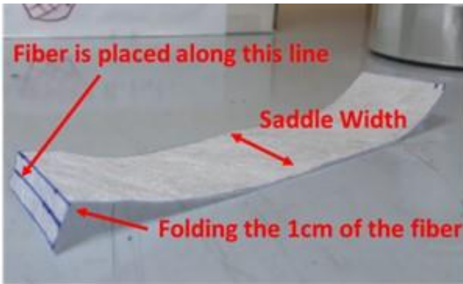
b) Cutting the paper and draw guidelines
