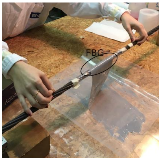
Figure 18. a) Putting the FBG sensor on the Polyester, and b) rolling the remaining part of the Polyester around the FBG sensor and strand.
