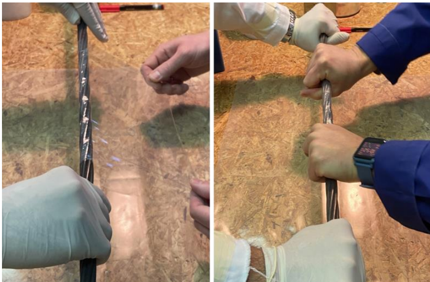
Figure 16. Coating the strand surface with plastic film.
