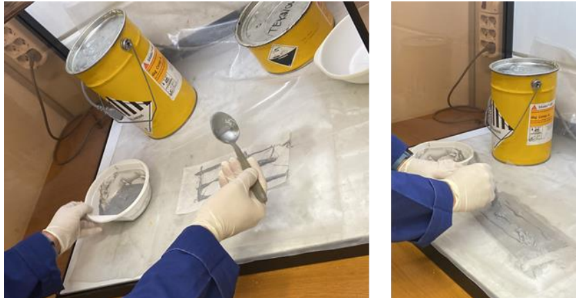
Figure 15. Putting the mixed epoxy resin on both side of Polyester.
