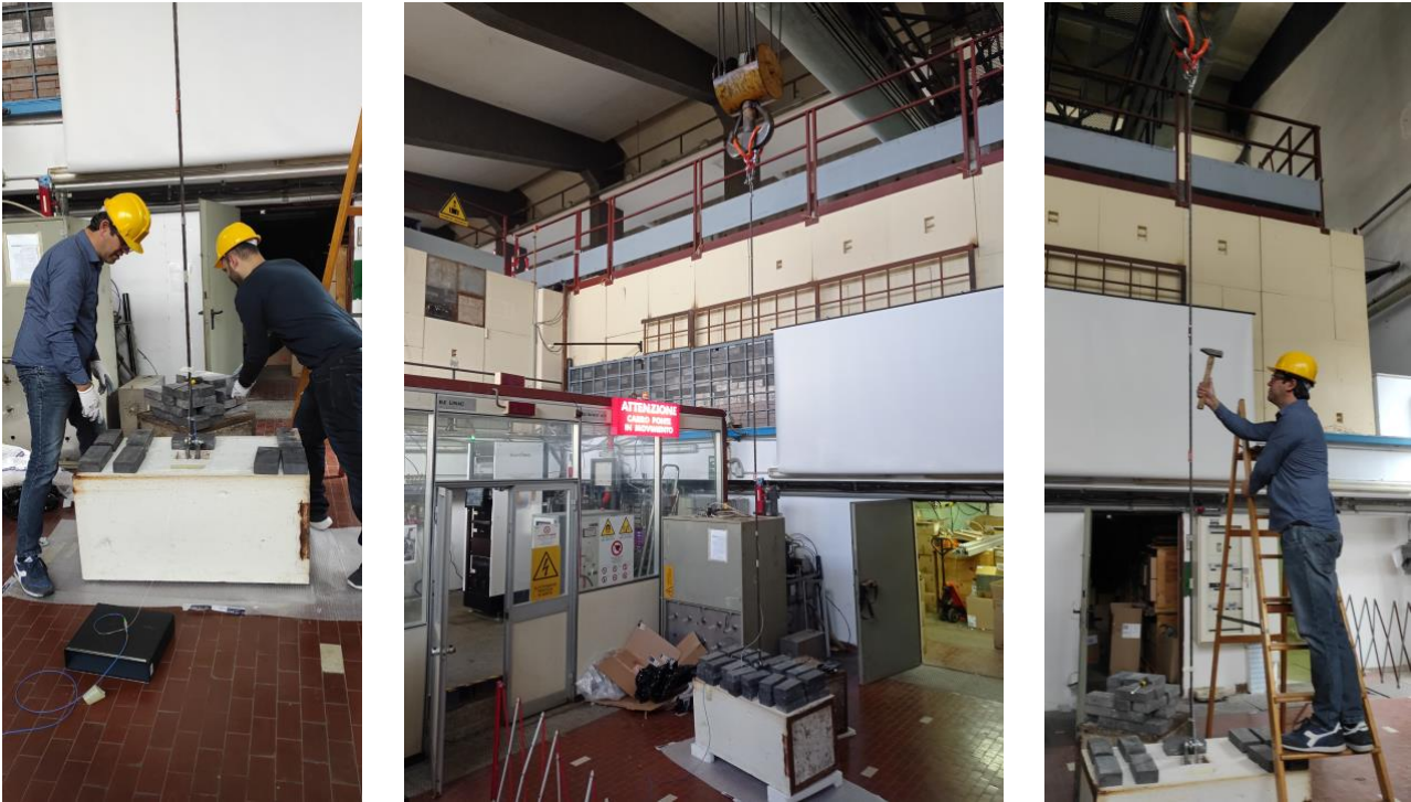
Figure 65. On the left: progressive increase in load using lead blocks heavy to the strand; in the middle: the overhead crane that supports tensioned cable; at right: dynamic test by striking with a sharp blow.
