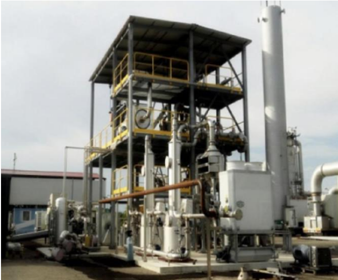
Figure 6 - Three staged gasification pilot plant
