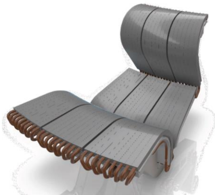
Fig. 1.6: DTT actively cooled divertor element (power input). This will permit experimental disruption study campaigns that could be even finalized to help ITER in getting all the necessary licensing.
