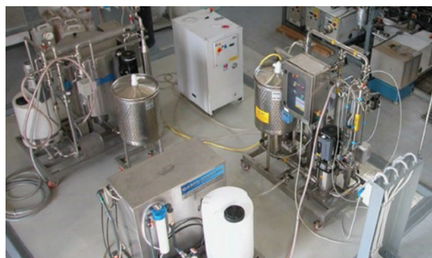
Figure 3. Selective fractionation of agro-industry and bio-industry wastewaters by ENEA membrane technologies
