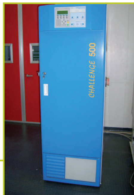
Specimens Maturing: Climatic Chamber Angelantoni Challenge CH 500 VP
