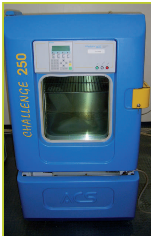
Cyclic Temperature Gradient Resistance: Climatic Chamber Angelantoni Challenge CH 250 C
