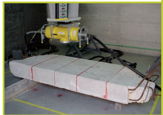
Radiographic facility 20÷450 kV, 5 mA
