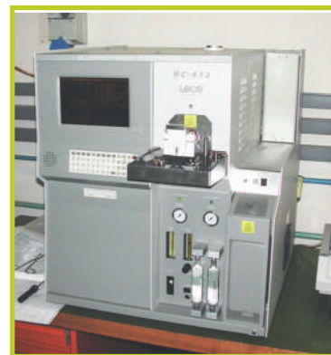
Modified version of hydrogen analyzer (LECO RC 412), one of the components of the prototype system for hydrogen embrittlement tests by means of in-situ electrochemical charging
