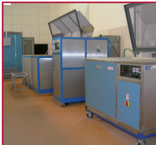
Climatic and salt-fog chambers for environmental qualification tests of nuclear components and systems
