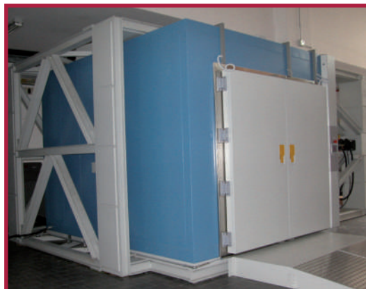
Climatic chamber for combined tests of thermal cycles, mechanical stress and UV irradiation
