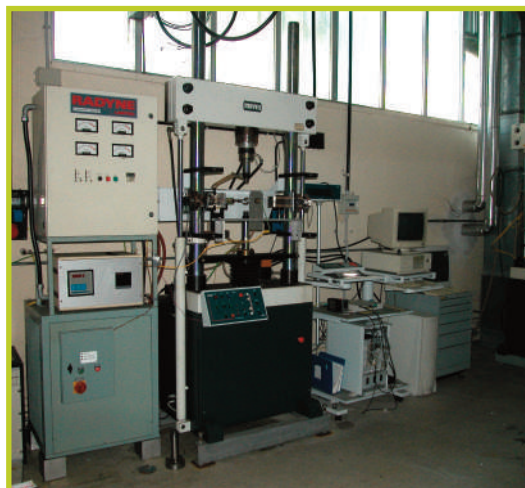
100 kN Mayes universal testing machine to carry out thermo-mechanical fatigue tests (inductive heating)
