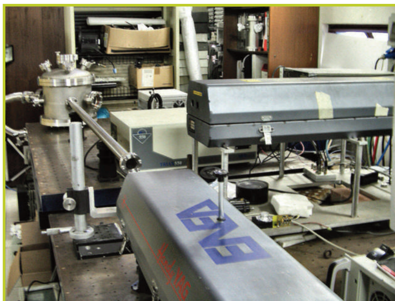
Transportable high-resolution LIBS system available at the ENEA Frascati Research Center; on the background, the chamber for remote analysis (2 m distance) of in-vacuum samples
