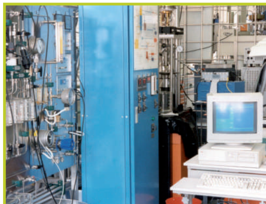
Recirculating autoclave circuit for mechanical tests in high-temperature pressurized water: view of the low-temperature circuit for water chemistry conditioning and control
