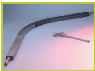
Copper tube with tungsten and CFC (Carbon Fiber Reinforced Carbon) tiles of the ITER divertor component
