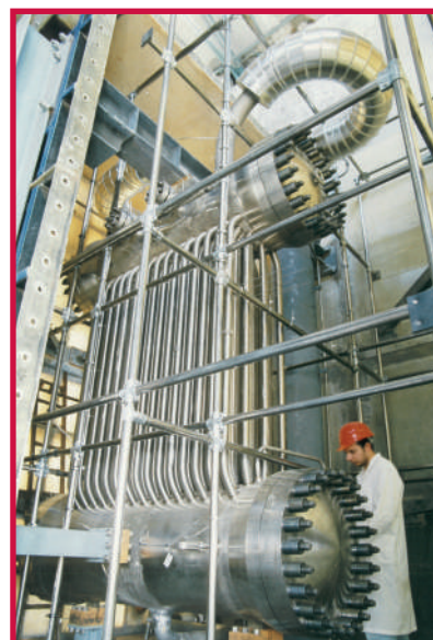
SBWR Isolation Condenser testing on the PANTHERS facility (power: 20 MW)
