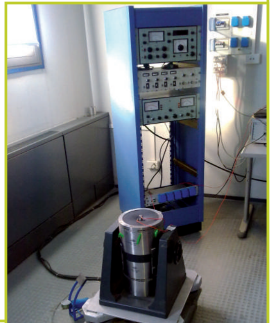
Traditional calibration system for accelerometers in the frequency range 10÷10,000 Hz
