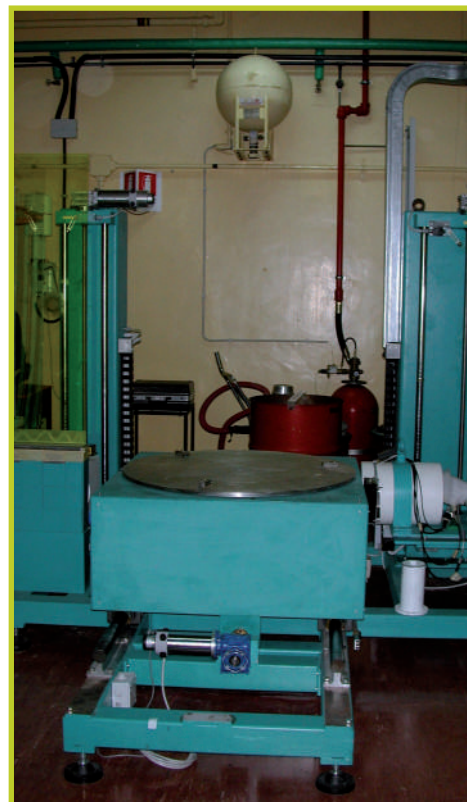
Measurements on drums containing gamma-emitting radionuclides: SRWGA System (Sea Radioactive Waste Gamma Analyser)
