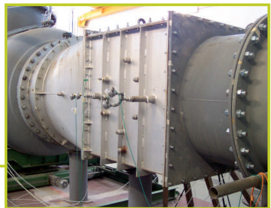
"External combustion" full scale component holder (gas duct section 600 × 600 mm)
