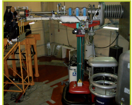
RadHard testing of FBG sensors at the Frascati Neutron Generator plant (ENEA – Frascati Research Centre)
