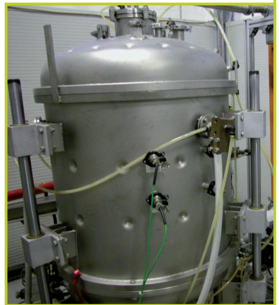
CVI (Chemical Vapour Infiltration) device for ceramic matrix composites
