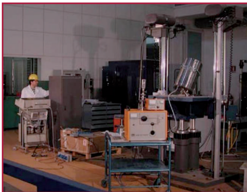
70 cm drop test of a container for plutonium solutions
