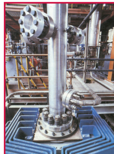
SPES-2 experimental facility: upper head of the power channel (power: 5 MW, n. 97 heated rods)
