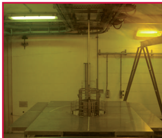
Irradiation cell and rack with 60 Co sources; in the foreground: platform for sample positioning
