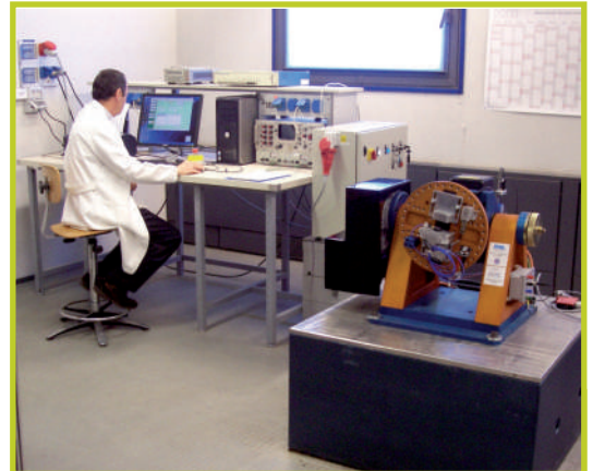
STASI System for accelerometer calibration in the frequency range 0.01÷10 Hz
