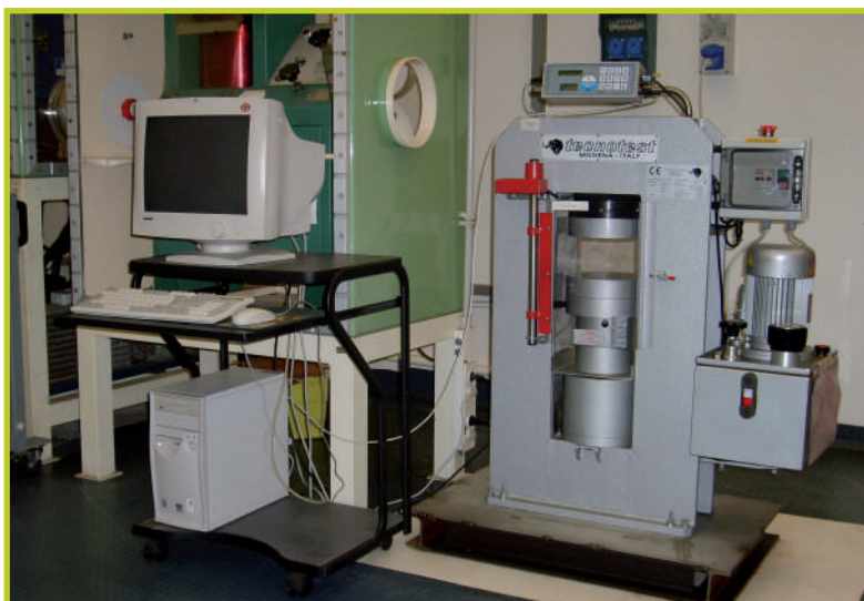
Compressive strength: Hydraulic Press Tecnotest KC 150
