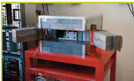
National standard for beta-gamma emitting nuclides activity measurement ( 4\pi\beta\text{-}\gamma system)
