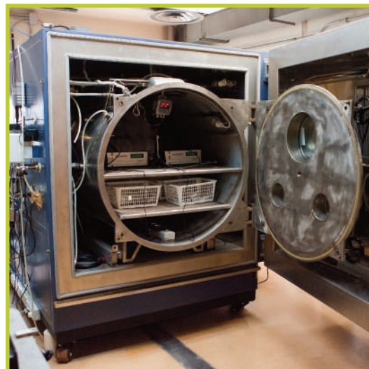
National standard for radon atmosphere reference dosimetry (radon chamber)
