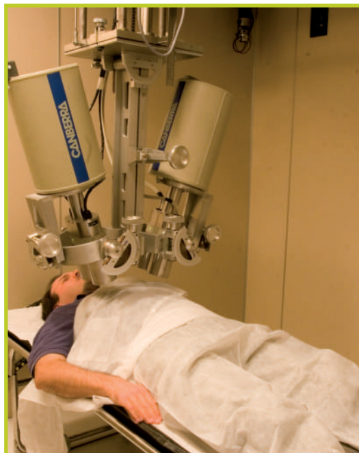
IRP Casaccia – Laboratory for in vivo measurements (Whole Body Counter, WBC): lung activity measurement for radionuclides emitting gamma rays from 10 to 100 keV
