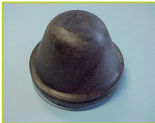
Alpha track radon passive sampling device (ENE A patent, MI2006A000703)
