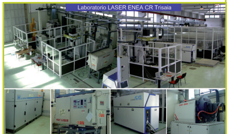
Views of the 400 m 2 Laser Hall: 4 working stations and 4 laser sources with nominal power ranging from 1.8 to 6 kW used in the development of welding and surface treatment processes and for fabrications of prototypes and small series
