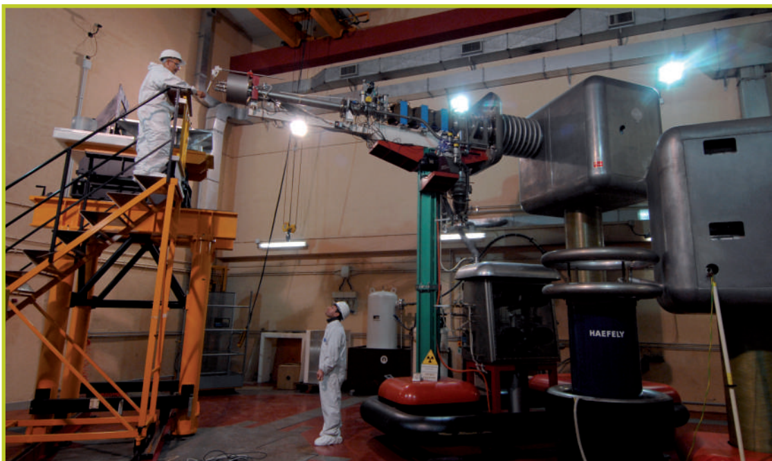
Preparing for irradiation of some samples to be activated by the neutrons produced by the FNG
