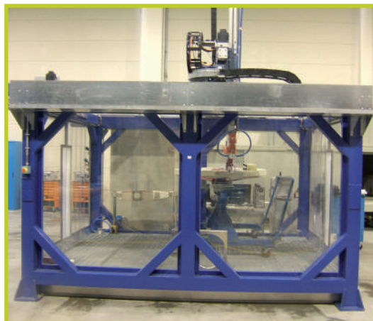
Automated 6-degree-of-freedom ultrasonic system for the aviation industry
