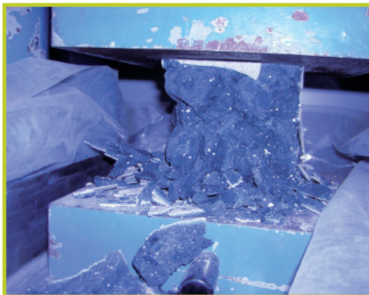
Compressive strength test
