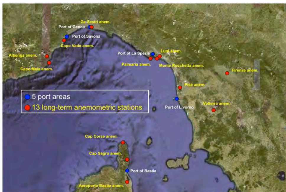
Figure 2: Map of the Northern Tyrrhenian Sea indicating the 13 long-term anemometric stations used to study the wind climatology of the 5 port areas.
