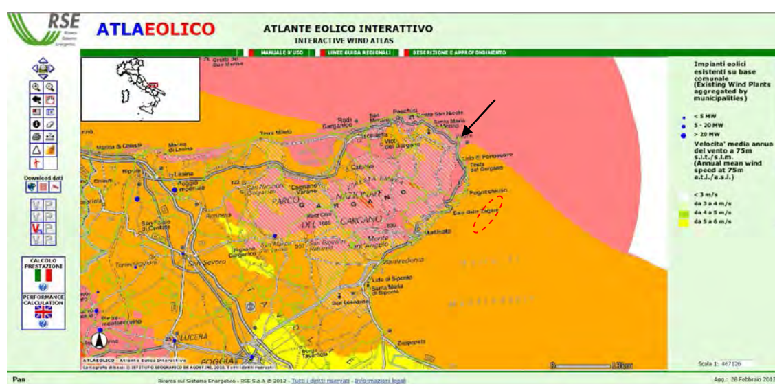
Figure 4: Annual mean speed map at 75 m a.g.l./a.s.l. in the area of Manfredonia Gulf: offshore wind plant area (red dotted line) and Vieste measurement station (black arrow).
