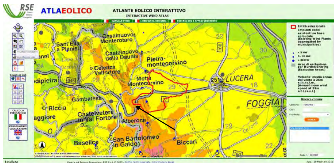
Figure 3: Exclusion area map (shaded zones), installed wind capacity (blue circles), Volturino municipality boundary (red line) and Volturino plant (black arrow).
