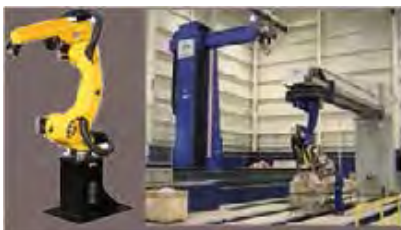
Figure 7: Inspection on aeronautical component with squirters and anthropomorphous robot.
