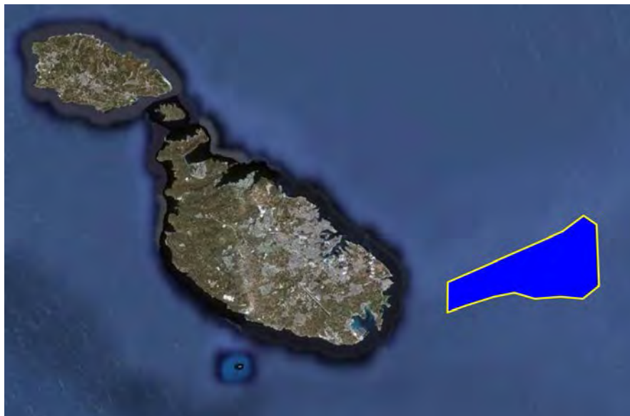
Figure 1: The South East Offshore Zone (SEOZ) outlined for the area having a maximum sea depth of 70 m.
