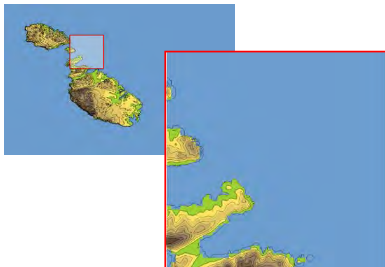
Figure 10: WindSim™ screenshot showing the extent of the Macro model and the Micro_01 domain.
