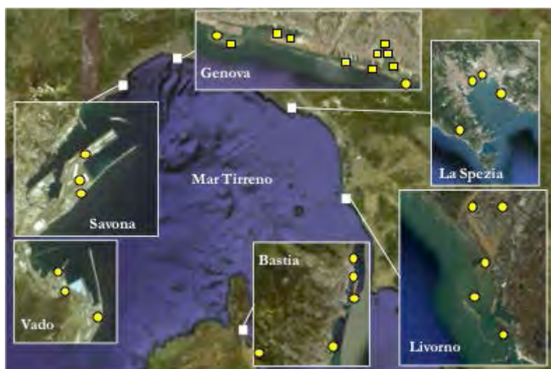
Figure 3: Anemometer stations installed in the 5 port areas: financed by the project (yellow circles) and by the Port Authority of Genoa (yellow squares).
