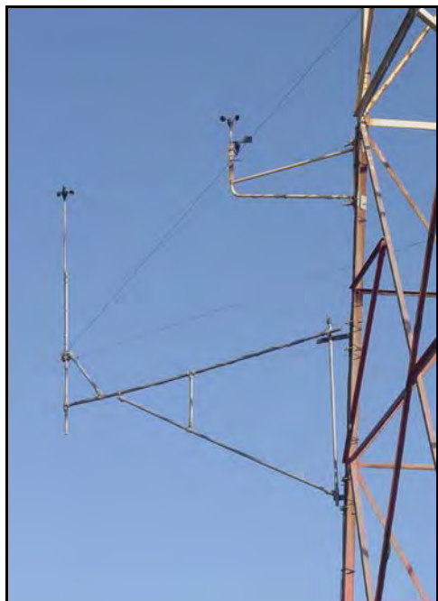
Figure 2: The 10 metre level sensor cluster at Wied Rini which is being used as a source for the long-term ‘donor’ dataset is shown on the short supporting boom close to the tower.
