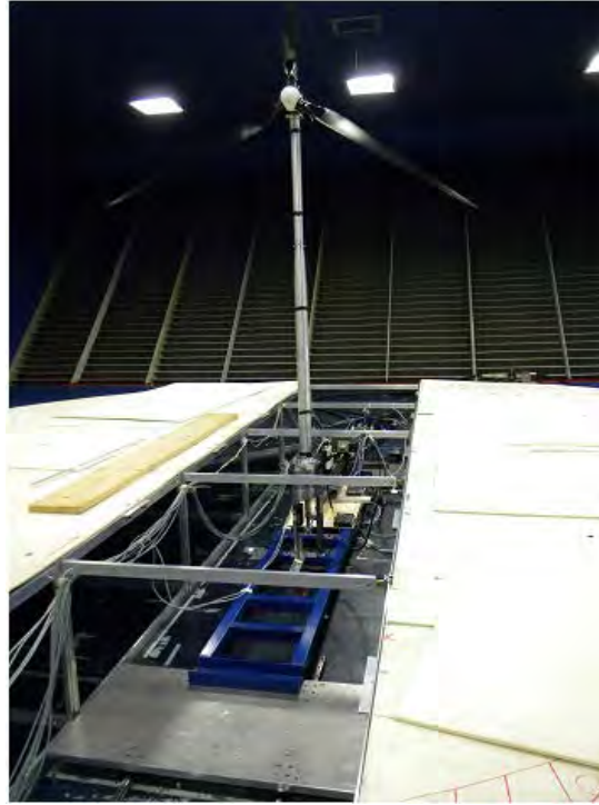
Figure 1: Wind turbine scale model on the test rig in the wind tunnel BL test section.
