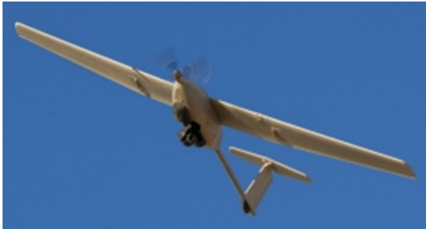
Figure 22. The Stalker, by Lockheed Martin, has a wingspan of about 3 m (10 ft), weighs about 6.4 kg, and it can be launched by hand, flying for up to two hours at up 4600 m altitude; in 2011 Lockheed Martin announced a new version of its Stalker called eXtreme Endurance (XE) powered by Ultra Electronics' industry-leading solid oxide fuel cell. [source: Lockheed Martin, www.lockheedmartin.com ]
