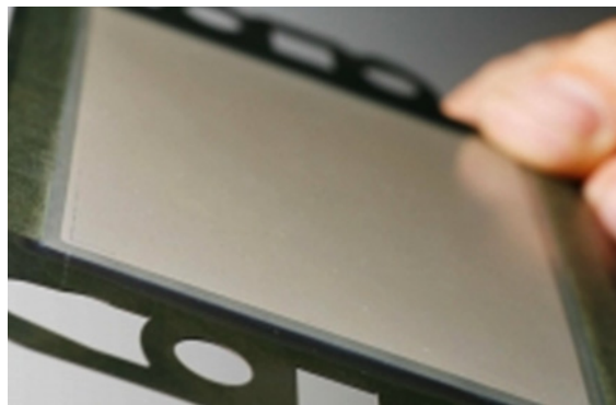
Figure 27. Detail of a Ceres' single fuel cell; electrolyte is sandwiched between the anode and the cathode and it is very thin.
