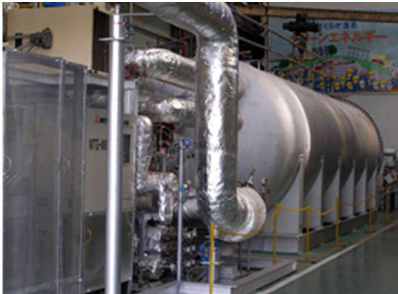
Figure 41. Mitsubishi's 200 kW coupled SOFC-microturbine system. [Source: MHI, Proceedings of Fuel Cell Seminar 2011]
