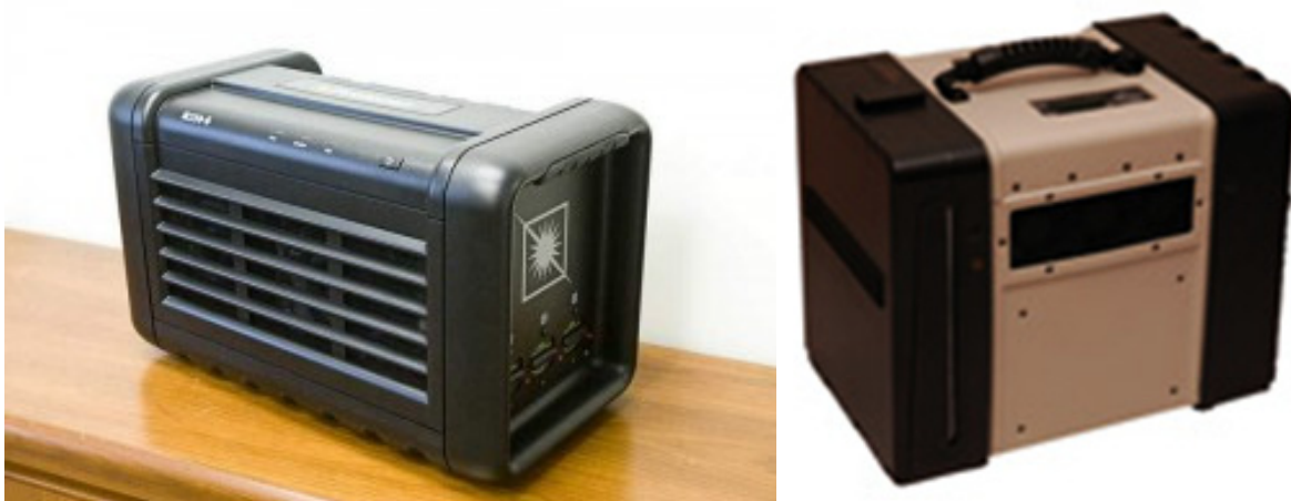
Figure 20. Protonex M250-B (250 Watts, up to 1000 operating hours, 2 hours/litre consumption, 38 dBA @ 7 meter, 18 kg weight, operating temperature from -20 °C to 50 °C, size 56x35x30 cm) and M250-CX B (300 Watts, 2000 operating hours, 900 ml/hour consumption @ 300 W, 38 dBA @ 7 meter, 16 kg weight, from -20 °C to 50 °C operating temperature, size 30x37x23 cm).
