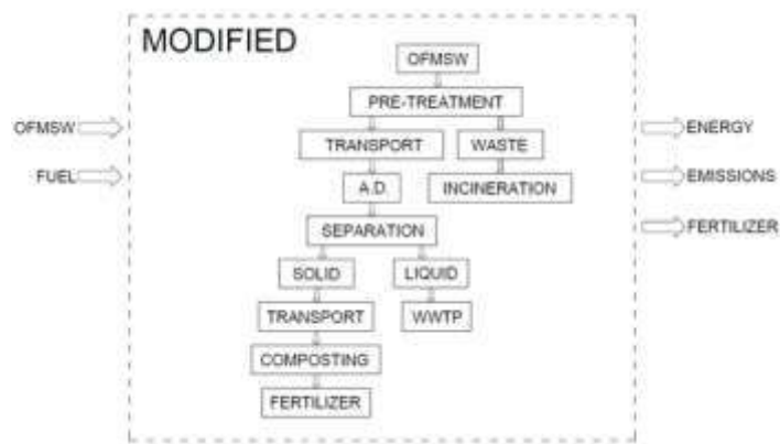
Figure 2: System boundaries and flow chart of the modified scenario.
