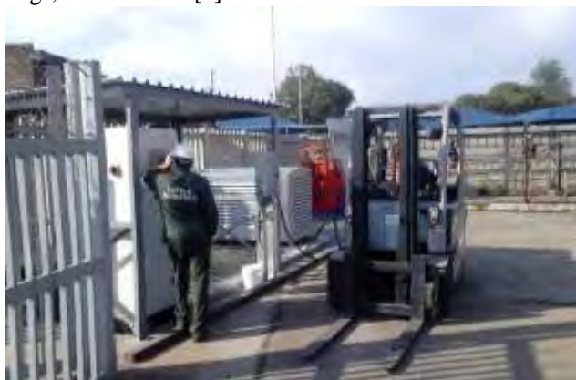
Figure 2. Refuelling of the fuel cell forklift with “hybrid” MH + CGH 2 hydrogen storage at Impala Platinum refineries
