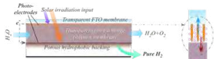
Fig. 1. Picture of the FotoH2 concept cell.
