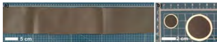
Fig. 1. Photographs of (a) the top view of the green tape and (b) complete cells.
