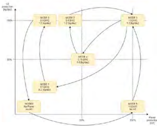
Fig. 1. CH2P operation points with laboratory testing scheme
