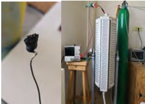
Fig.1a Electrolysed carbon, Fig.1.b Electrolysis process
