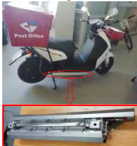
Figure 3. Fuel cell scooter (top) with MH hydrogen storage tank (bottom).
