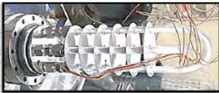
Fig. 3 Coolant channels with cooling fins.
