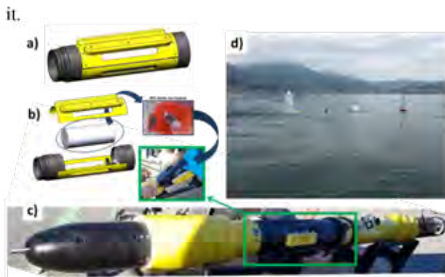
Fig.1. a) 3D-render of the MFC-payload, b) the open payload, with pictures showing the s-MFC assembly, c) the final AUV-Glider system with the newly MFC-payload, d) a picture taken during tests in seawater.
