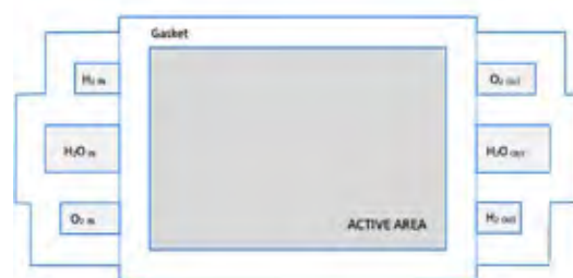
Fig. 1. Bipolar plate configuration used for the parameterized model
