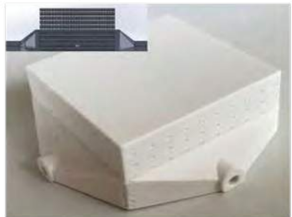
Fig. 2. SOFC stack prototype 3D printed. Onset: Model of the prototype.
