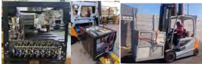
Figure 1. Left: frame of the power module with installed MH tank (bottom) and gas buffer (top left). Middle: installation of the assembled power module into forklift compartment. Right: VDI2198/VDI60 tests of the forklift with the power module
