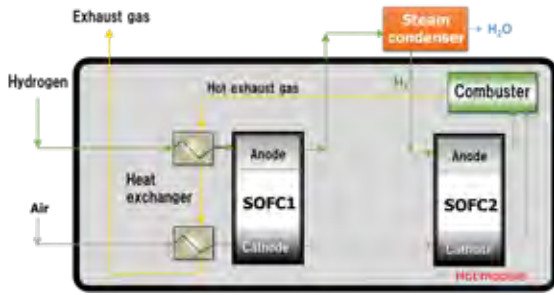
Fig.1. The schematic illustration of system flow of the hot module.
