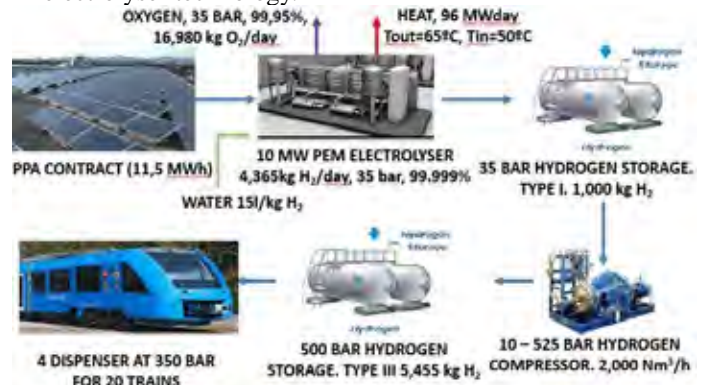
Figure 1. Trains Hydrogen Refueling Station.
