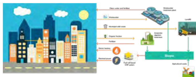
Fig. 1. Waste-to-energy circular approach with high temperature fuel cell-based cogeneration systems.
