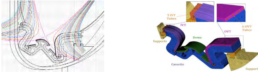
Figure III.11: Design of the reference initial divertor for the proposed DTT. The left one is a conceptual one. The right one is the first draft actual design.
