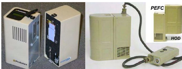
Prototipi 30 W (P1 e ProPack 50) – Protonex/Millennium Cell
