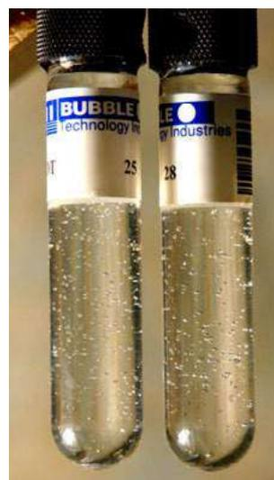
Fig. 6. The BDT detectors after neutron generation
