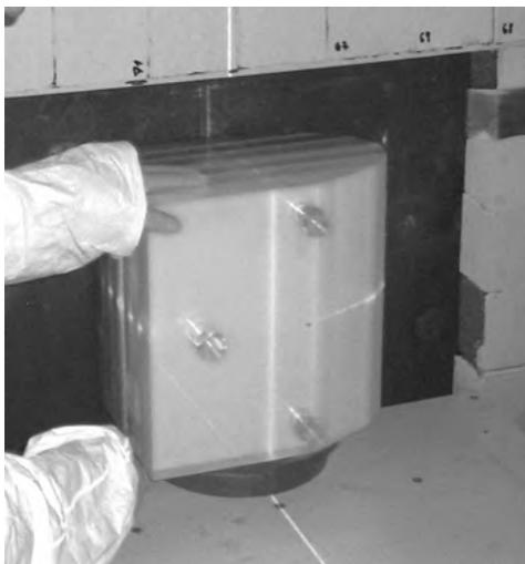
Fig. 6 – Phantom placed against the collimator exit of the LVR-15 BNCT epithermal column
