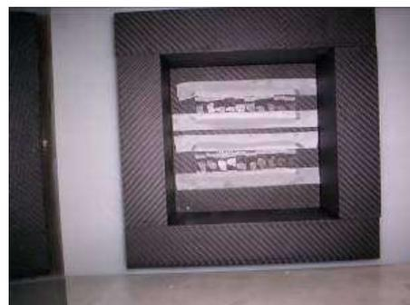
Fig.8. Biological sample positioning inside the irradiation cavity
