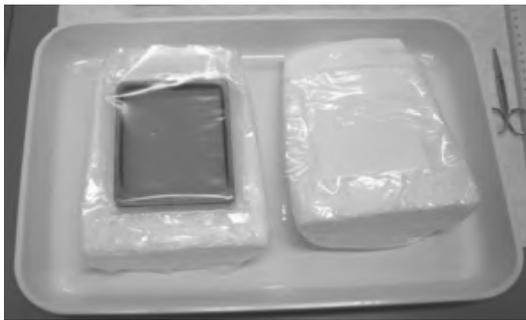
Fig. 5 – Lung phantom cut in the vertical plane, in which gel dosimeters were placed
