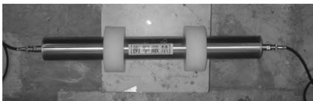
Fig. 3. Photo of the prototype low energy neutron spectrometer. A BNC connector is seen in both ends of the spectrometer.
