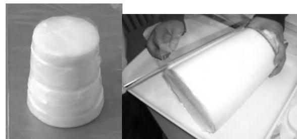
Fig. 4 – Lung phantoms, cut along (a) three horizontal planes and (b) one vertical plane, in order to place dosimeters.
