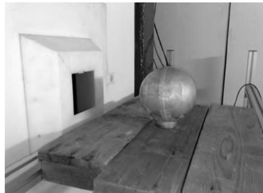
Figure 2. One of the Bonner spheres located in front of the beam aperture
