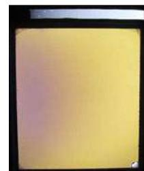
Fig. 7. Gel dosimeters after irradiation, placed on the light source for transmittance image detection
