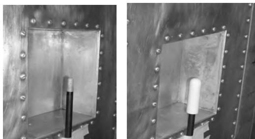
**Figure 1.** Bare ionisation chamber (left) and ionisation chamber with Li-6 cap (right) in the centre of the thermal neutron beam at the LFR Petten
