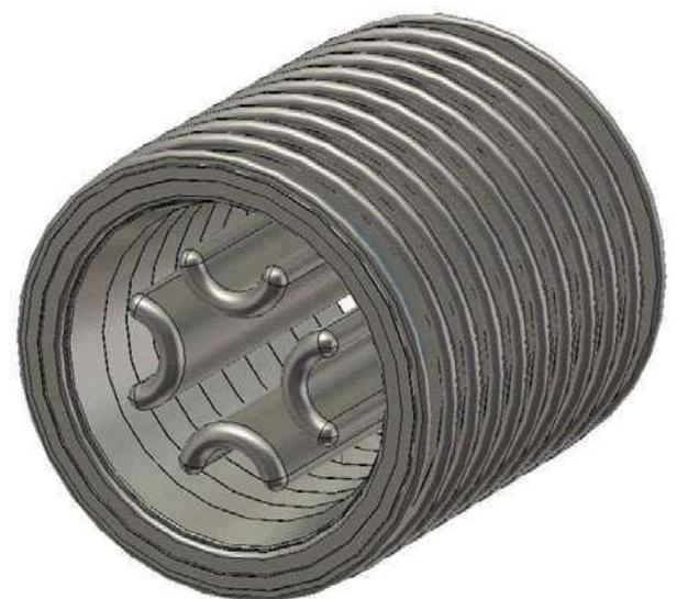
Fig. 4 View of an entire tube section showing all four quadrupole electrodes
