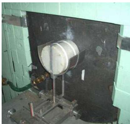
*Fig. 1. The cylindrical water-equivalent phantom put closed to the beam mouth. Two  $16 \times 14 \text{ cm}^2$  dosimeters are inserted vertically on the cylinder axis*
