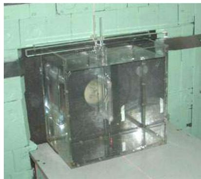
*Fig. 2. A couple of  $16 \times 14 \text{ cm}^2$  positioned in the  $50 \times 50 \times 25 \text{ cm}^3$  water phantom. The beam aperture (d: 12 cm) is visible*
