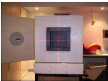
Fig.1. The neutron photoconverter prototype
