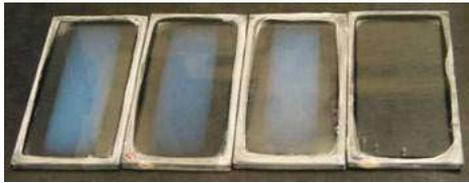
Fig. 1. Layers of polymer gel after irradiation
