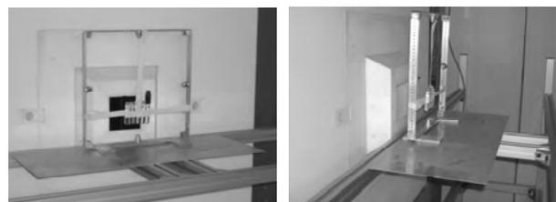
Figure 3. Bubble detectors located in front of the beam aperture (left) and 10 cm far from the aperture (right)
