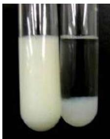
Fig. 1. Appearance of Gd-nanoCPs before (right) and after (left) coating with soybean lecithin
