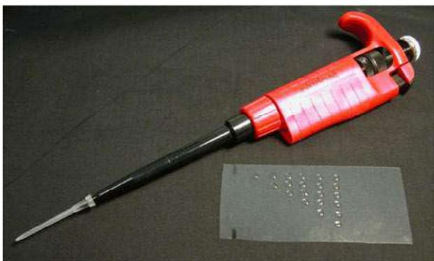
Figure 3. Photo of the micropipette and of a typical sample with columns with a different number of spots
