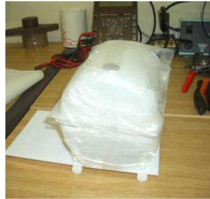
Fig. 2. Phantom utilised for the irradiation of gel dosimeters layers
