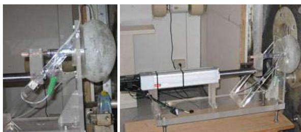
Figure 1. The self-made ellipsoidal head (Snyder) phantom (left), and the servo motor system (right)
