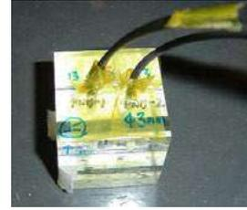
Fig. 4. Acrylic box and SOF detector
