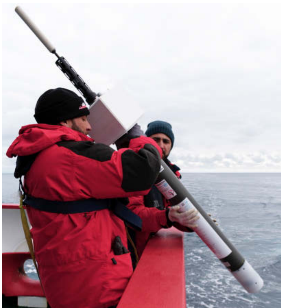
Prog. 2016/B2.01: Yuri Cotroneo and Pasquale Castagno deploying an ARGO float from the S/A Agulhas II
