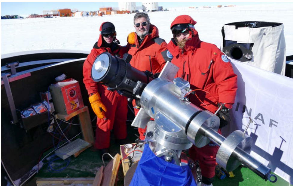
Prog. 2015/AC3.02: AntarctiCor telescope mounted on ASTEP system
