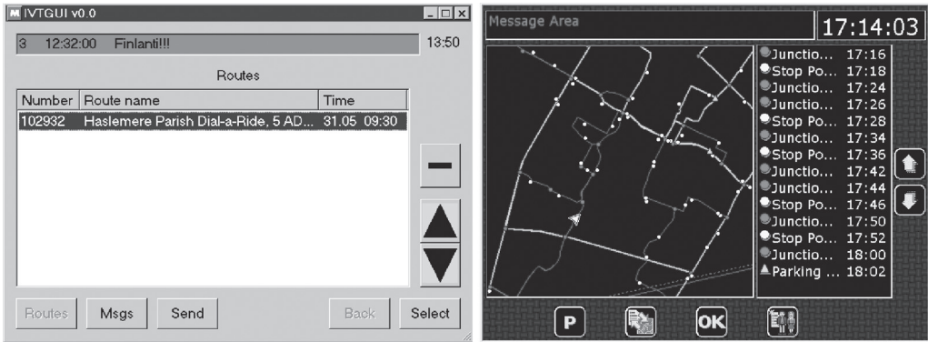
Figure 5.4: User interface of the DRT applications for the INVETE in-vehicle terminal for Finland (left, Mobisoft) and Italy (right, Softeco Sismat)
