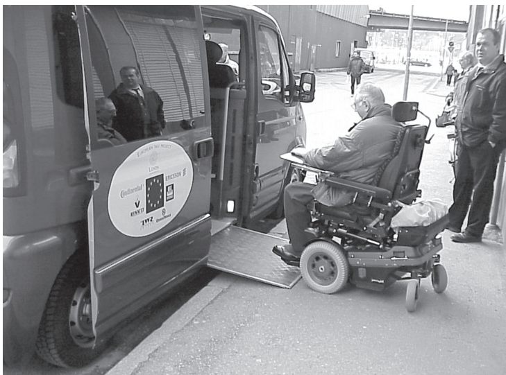
Figure 6 .7: Wheelchair user boarding the prototype vehicle with minimum assistance from the driver
