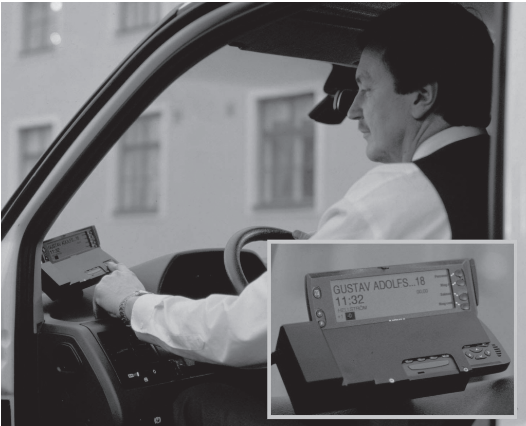
120 Figure 5.2: Nokia Communicator 9110 used as SIPTS in-vehicle terminal
