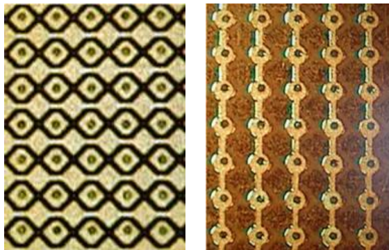
Figure 1. Microscopy picture of the anode layout; on the left: (pad side), on the right: back (strip side).
