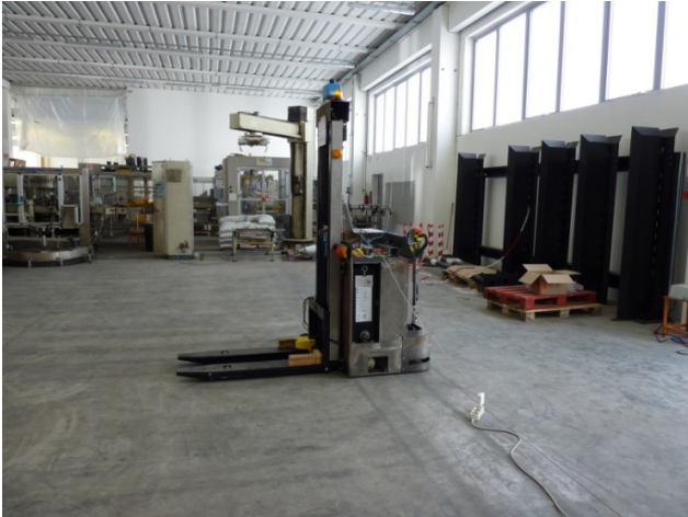
Fig. 36 - A prototype of automatic guided vehicle
