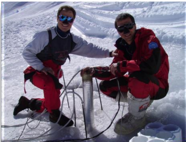
Fig. 63 - PANDORA a subglacial navigation robot designed by ENEA for Antarctica national program- tests on alpine glaciers
