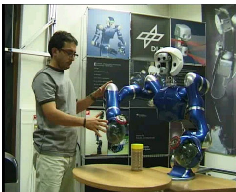
Fig. 74 - Manipulator developed in the Phriends project
