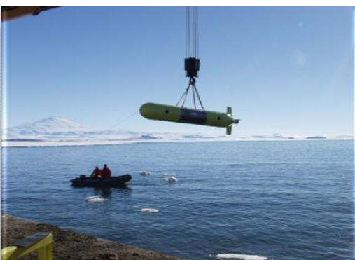
Fig. 57 - SARA (on the top and aside): the first “Sottomarino Antartico” Robotizzato” at ENEA
