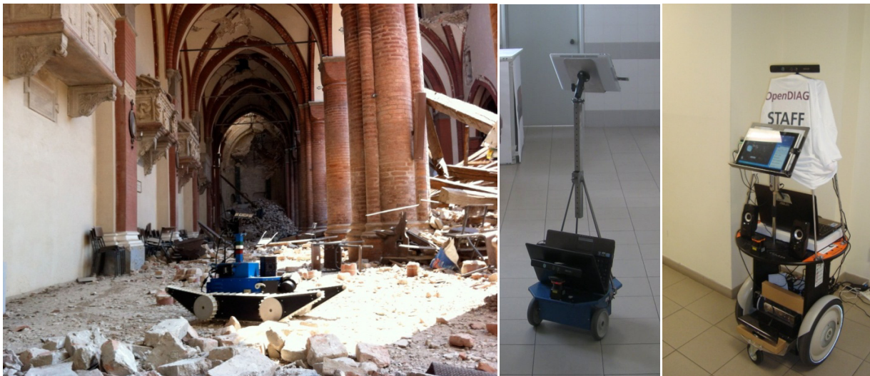
Fig. 68 - (Left) The TALOS mobile robot in field operation after the earthquake in Mirandola, and Social robots for Smart Monitoring of Complex Public Scenes (center and left)
