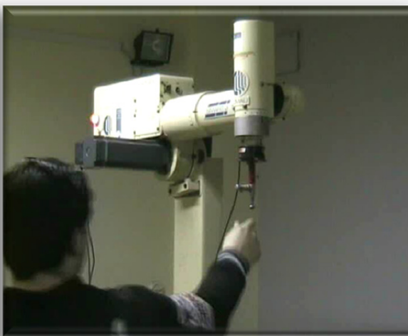
Fig. 72 - COMAU Smart 3-S robot with Open control architecture, ATI force/torque sensor and 6-DOF spatial impedance
