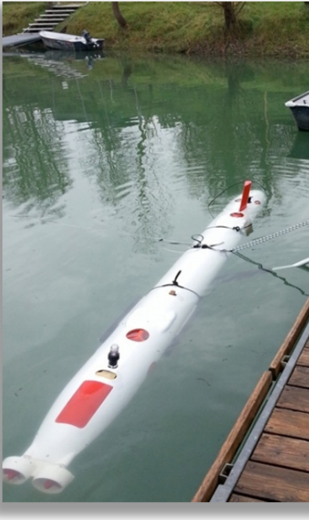
Fig. 51 - Tifone, vehicle for sea bottom patrolling designed by Piaggio Institute
