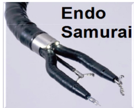
Fig. 29 - Endoscopic robot for surgery
