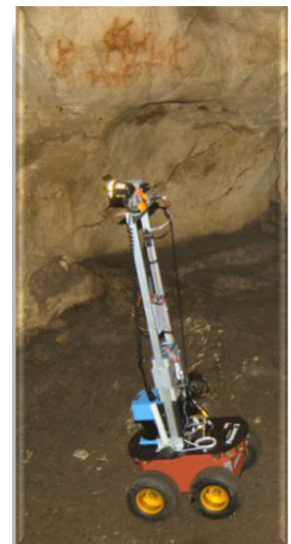
Fig. 77 - Robot used for cave exploration
