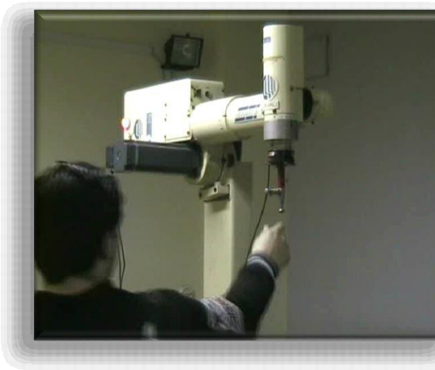
Fig. 72 - COMAU Smart 3-S robot with Open control architecture, ATI force/torque sensor and 6-DOF spatial impedance
