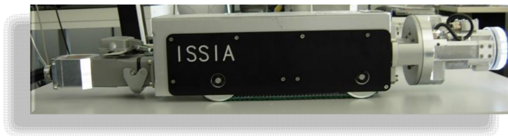
Fig. 78 - Prototype of mobile robot for non-destructive inspection of a multispar structure of Boeing 787
