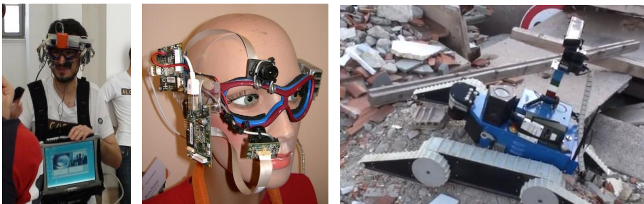
Fig. 66 - Research activities at ALCOR Lab: Eye tracker (left) and Gaze machine (center) for experiments on visual localization and recognition; TALOS robot moving on harsh terrain in a firemen training field (right)
