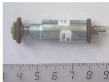
Fig. 1 Miniature in-tube robot.
