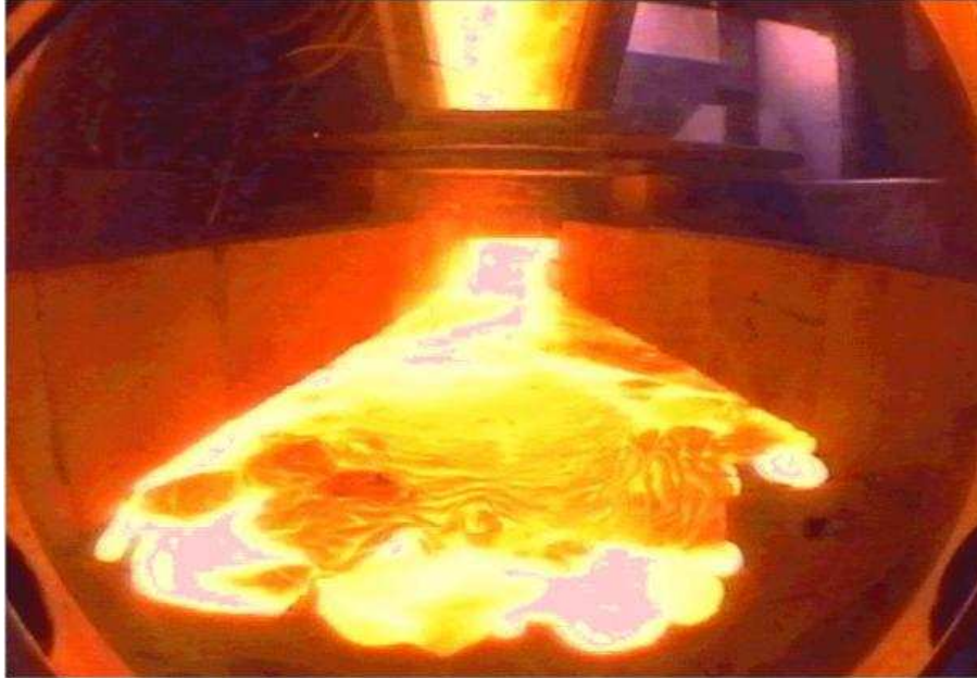
Figure 1: Corium spreading test at the French CEA VULCANO facility (UO 2 with some ZrO 2 ) ( http://www.iaea.org/NuclearPower/Downloads/INPRO/Files/2010-Feb-DF-WS/15-Teller.pdf ).
