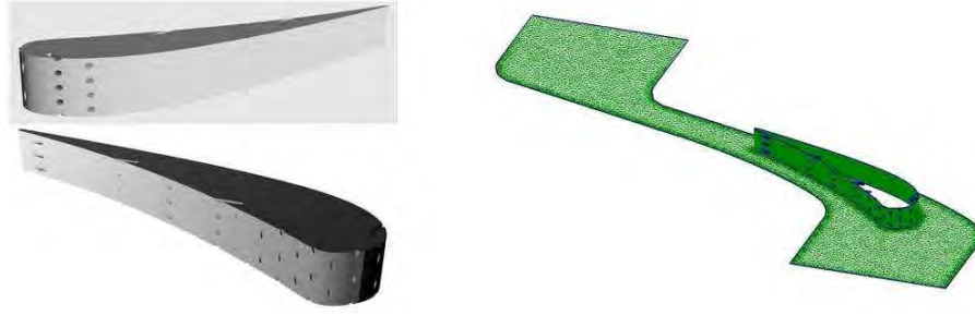
Figure 3: a) EEE blade vane-vane profile; b) EEE blade vane-computational domain with cooling holes.
