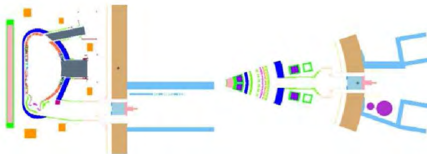
Figure 2: ITER B lite v3 MCNP model upgraded with the Lower Port #12. Poloidal section along the Cryopump longitudinal axis (left) and toroidal section along the Cryopump mid-plane (right).
