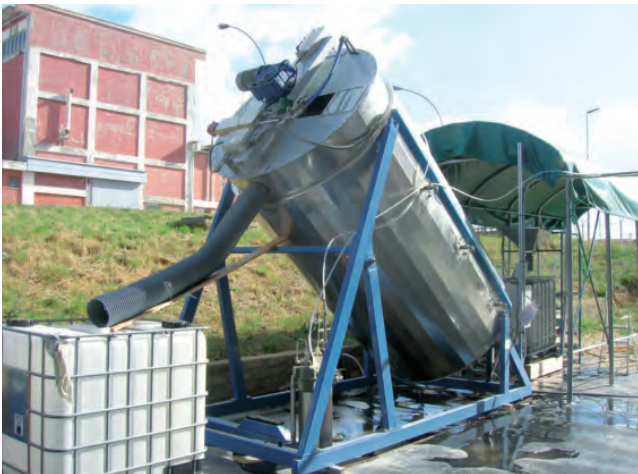
Mobile anaerobic digester
