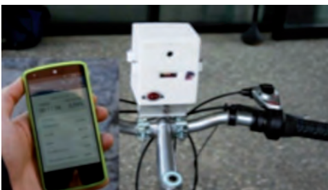
MONICA prototype mounted on a bicycle and its App screenshot for Android smartphones
