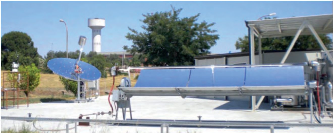
ENEA Trisaia test facility for the characterization of concentrating collectors at medium temperature
