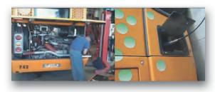
After the very positive results certified by the homologation test at the Institute for Research on Engines in Naples, the engine was mounted on board **MHYBUS**, a bus that provides public transport in Ravenna using a 15% hydrogen mixture available at the SOL plant, using an easily transportable gas compression station (an 8-meter container) owned by ENEA.
