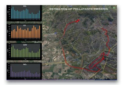
**ECOTRIP©** is a software that can accurately calculate fuel consumption and exhaust emissions (carbon dioxide, carbon monoxide, nitrogen oxides, volatile organic compounds and particulate matter) thanks to on-board units connected to an operation centre.
