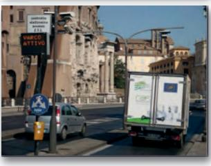
**EFRUD** is an innovative transport system for perishable goods that reduces the environmental impact and improves the energy efficiency of this business. Financed under the European Commission's LIFE + programme, it uses a refrigerated cell based on the storage of frigories (without the use of a compressor) and mounted on dual mode vehicles (electric/diesel) that can operate using the thermal engine in the extraurban areas and the electric traction within the city.
