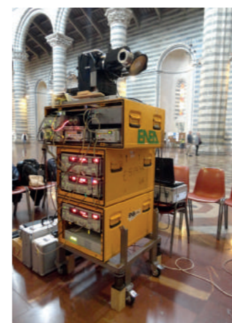
Crack analysis of Orvieto Cathedral by ITR laser technology
