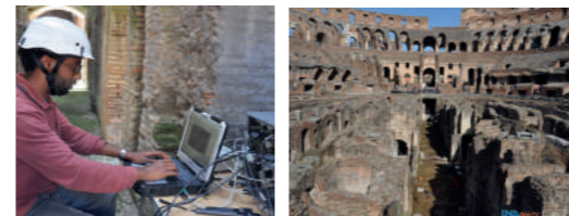
Monitoring of traffic-induced vibrations of the Colosseum
