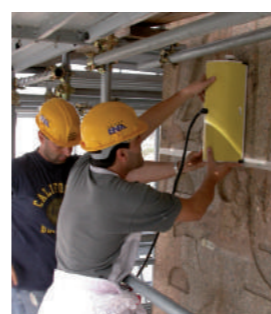
Structural tests of the Egyptian obelisk in Piazza San Giovanni in Laterano
