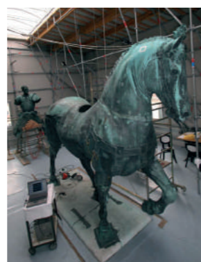
Monitoring by fiber optic sensors. Equestrian Statue by Bartolomeo Colleoni
