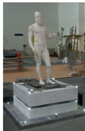
The Bronzes of Riace, antiseismic basement test on shaking table
