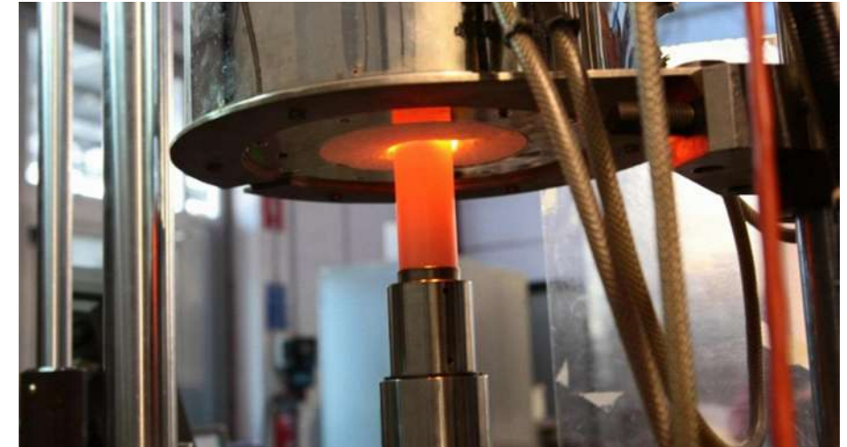
Thermomechanical tests on high temperature resistant materials (up to 1500 °C)
